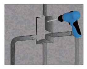
2. The depth of the embedded box is 2.2"-2.6". It's better to drill the depth of 2.2"for blank wall.
