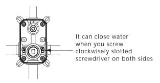
Note:If only colse one side that it will cause faucet abnormal outlet water,for normal outlet water please make sure the adjusting position on both sides is open(counterclockwise to open).
